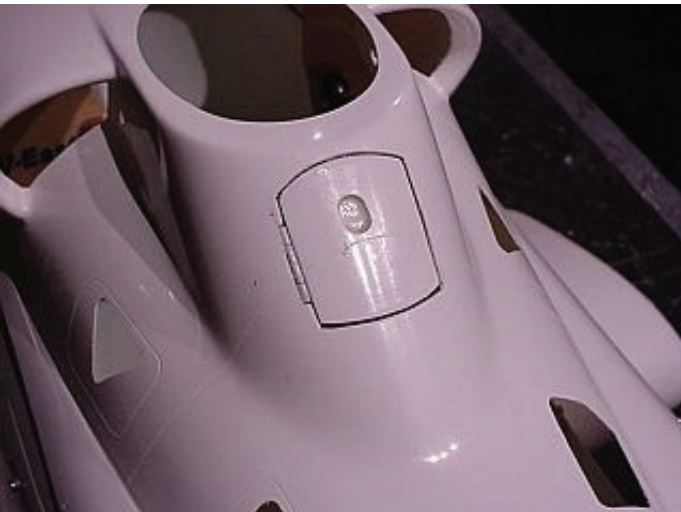
Hinge added , hole will be filled . This allows plenty of room for starting . Side screens and dome opening supply cooling air .
