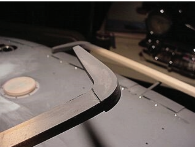
Running/step boards are 15 mm wide, 6 mm thick as per scale. 1/64 ply adds to build up the front step attachment point, two layers. Boards are 18 3/8" long.
