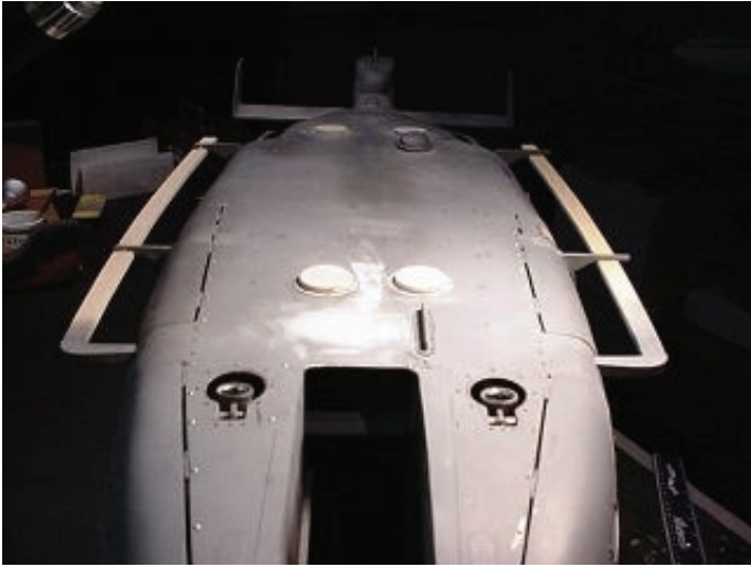
Nice full shot... #00 brass screws ground down to form pan rivets.
