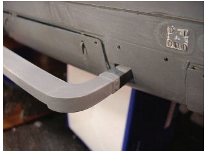
Nice full shot... #00 brass screws ground down to form pan rivets.
