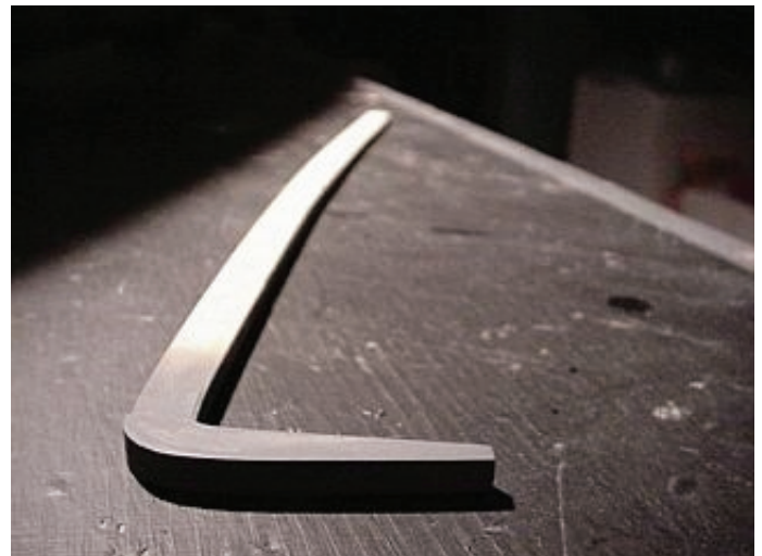
Running/step boards are 15 mm wide, 6 mm thick as per scale. 1/64 ply adds to build up the front step attachment point, two layers. Boards are 18 3/8" long.
