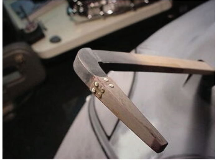
Nice full shot... #00 brass screws ground down to form pan rivets.
